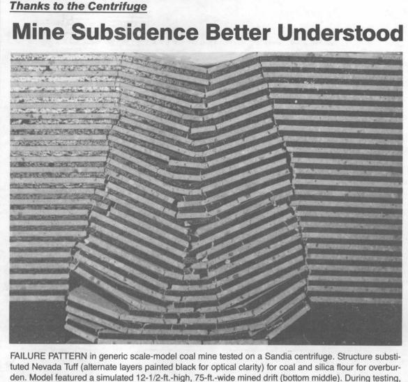
earth collapsed into the drift, causing signifcant subsidence of the scale model's surface.
